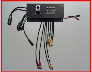
It **PREVENTS** the possibility of connecting errors during shooting because all the wiring is pre-assembled inside the case.
